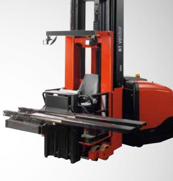
Man-down VNA truck suitable for pallet handling in medium-intensity operations. Turret head forks or high speed slidethrough fork versions
